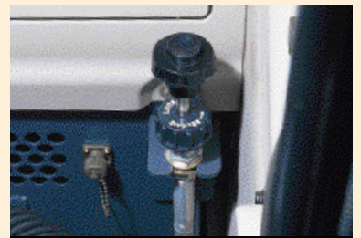
Emergency throttle cable
